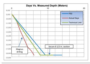
left compares estimated and actual drilling performance. The Magnus RSS (red line) finished drilling 41 hours faster than the customer's technical limit for an 8 1/2-in. well section (green line). It drilled 3 days faster than the P50 estimate for mid-range performance (blue line).
